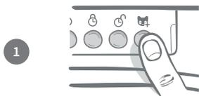
1 Remove the button cover to reveal the six buttons on the front of the Pet Door. Press the 'Add a pet' button once to activate the 'Add a pet' mode.
