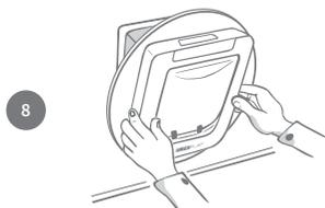
We advise that there are two people present for this step; one person inside the house and one outside. From inside the house, put the tunnel through the hole in the door ensuring it is going through the **centre of the hole and not touching any edges**. Remember the **SureFlap logo** and **LCD display** must be **inside the house**.
