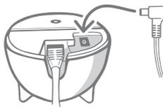
**Assemble the power supply** and plug it into your power outlet. Plug the other end of the cable into the base of your Hub.
