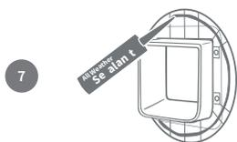
Apply a line of clear all-weather sealant to the back of both mounting adaptors, about 15mm ( $\frac{5}{8}$  inch) from the edge. Make sure your Pet Door is nearby and ready to be fitted. Place one of the mounting adaptors (it doesn't matter which) over the tunnel of the Pet Door so that the patterned side with the ribs is facing outwards and is not touching any surfaces.
