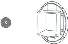
Place one of the mounting adaptors (it doesn't matter which) over the tunnel of the Pet Door so that the side with the sealant is facing outwards and is not touching any surfaces.
