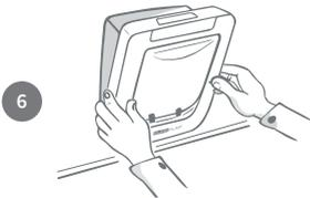
Now put the tunnel of the Pet Door through the hole. Remember the **SureFlap logo** and **LCD display** must be **inside the house**. We advise that you have two people for this, one inside the house and one outside to help hold the product firmly in place.
