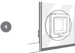
From inside the house, put the tunnel through the hole in the glass making sure the Pet Door is positioned centrally within the hole. Press firmly on both the Pet Door and the mounting adaptor so that you compress the sealant against the glass.
