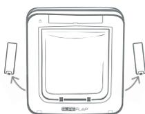
Remember that there are battery compartments on both sides of the Pet Door and that these will both need to be accessible once it's fitted.
